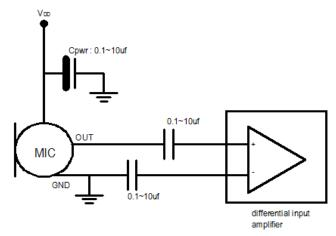
Figure 5. Recommended interface circuit for customers' applications
