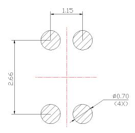
Figure 4. Example solder stencil pattern
