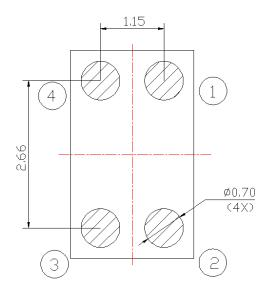
Figure 3. Recommended landing pattern on customers' PCB
